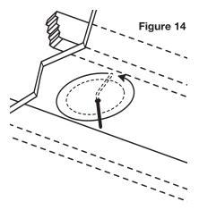
about an inch below the center of your proposed speaker location. BE VERY CAREFUL NOT TO DRILL THROUGH EXISTING WIRES, PIPES, OR STRUC-TURE. IF YOU FEEL ANY EXTRA RESIS-TANCE AS YOU ARE DRILLING, STOP.
